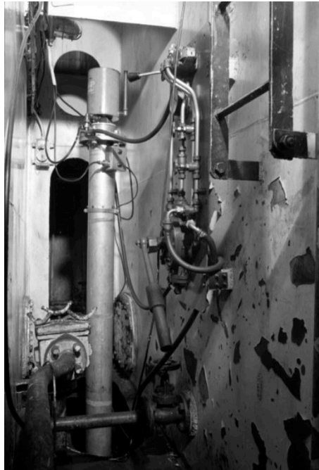
Figure 7. The Colnbrook EM Log spar (vertical tube just left of centre) on RRS Discovery was deployed and retracted using a hand pumped hydraulic system (large lever in the middle, with the small lever above to select up or down). Courtesy National Oceanographic Library/NOC, NOL archive 4619/2.
