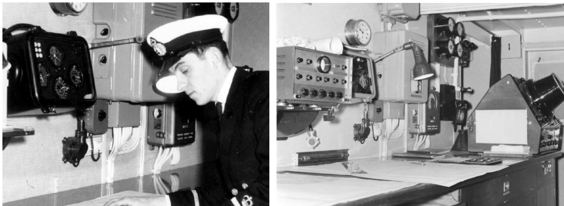
Figure 1. Chart Room of RRS Discovery . Left: in 1963 with a Decca Mk V decometer indicator dial. Right: in 1971 with, on the left above the chart table, an Enac Triton DX Navigator combined LORAN-A and LORAN-C receiver. Everett Sarratt, the designer of this equipment, had been presented with the inaugural Product Award of the US National Marine Electronics Association (NMEA) in 1964. Partially visible to the right of the LORAN receiver is a Decca Mk XII decometer readout unit. Courtesy National Oceanographic Library/NOC, NOL image 3197.
