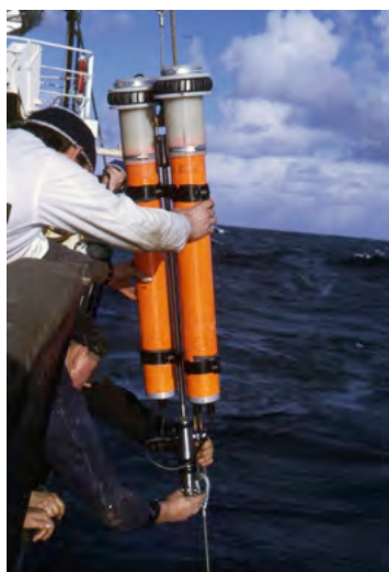
Figure 1. A pair of NIO acoustic releases with magnetostrictive nickel scroll transducers being deployed on RRS Discovery cruise 38 in early 1971, courtesy Raymond Pollard.
