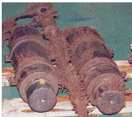
Figure 8. Pair of heavily fouled CR200 releases recovered by FS Alliance, 1992.
