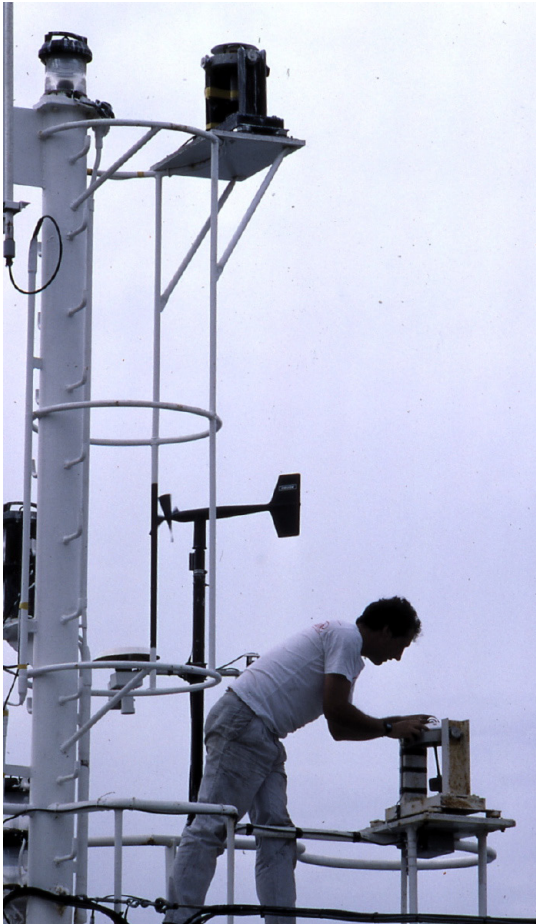
Robin Pascal cleaning a gimballed short-wave radiation sensor on the mast on RRS Charles Darwin. At centre there is a RM Young propeller-vane anemometer.
