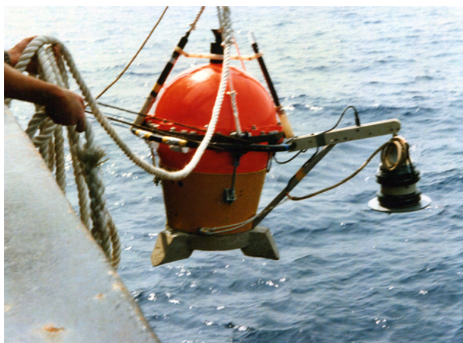
Figure 5. A DOBS fitted with an external 3-component geophone package being deployed during RRS Charles Darwin cruise 75 in 1993.
