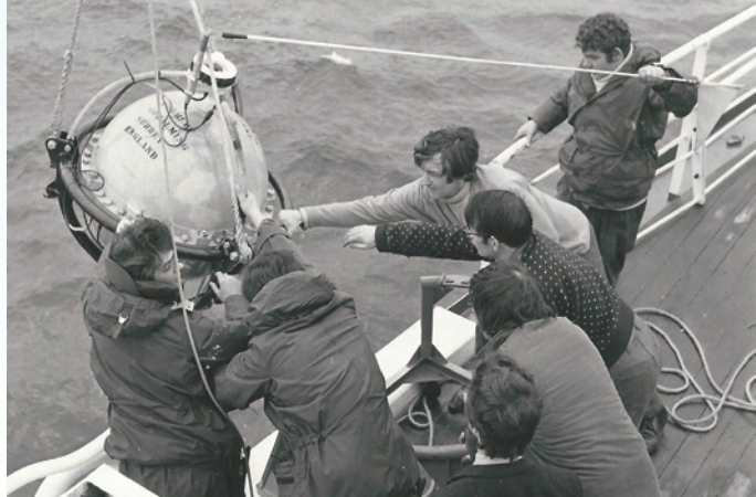
A PUBS Mk.I being recovered by the crew on the fore-deck of RRS Discovery. Note the broken radio aerial. Jack Langford and Bob Whitmarsh are second and third from the right.
