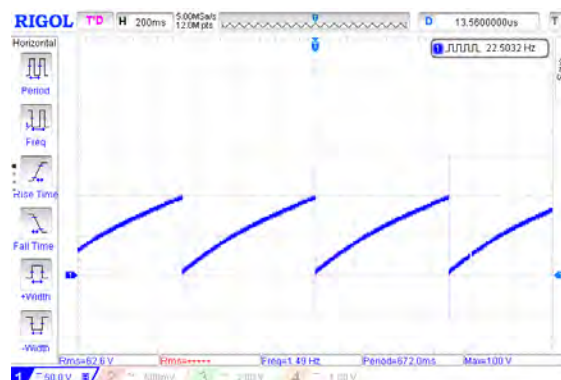
Figure 8 Voltage waveform at the trigger electrode. 200ms and 50V per division.
