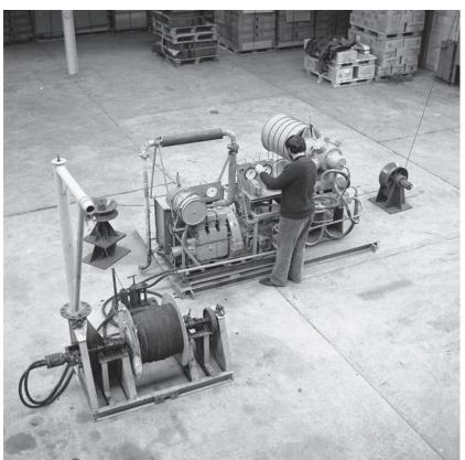
site that was frequently passed by ships en route to the N Atlantic). What was needed was a better winch that could handle a 1 ton load, would handle the shackles and connectors between wire lengths and ideally that could be transferred from ship to ship.
