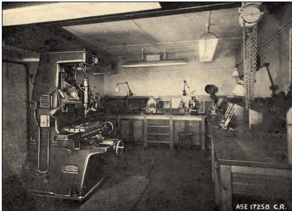
Figure 9. The Air-conditioned, temperature controlled workshop, with, left a jig borer that was used to position holes, or to check the location of holes, over an area of 36" by 24" to 2/10,000 of an inch, or to half a minute of arc on a circle of up to 16" diameter. The quill of a jig borer only moves in the vertical plane, achieving a greater accuracy over a conventional mill. ASE image 17258 CR from Backroom Window 4
