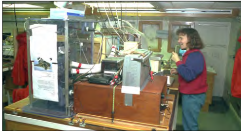
Richard Bellerby monitoring the operation of his pH measuring analyzer and Jane Robertson with her apparatus for p\text{CO}_2 measurements.
