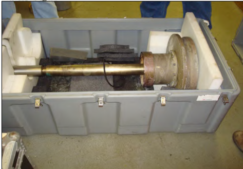
The phased array transducer for the acoustic Doppler current profiler in its transit case, and then in place on the inside of the ship's hull. After the transducer has been put in place, the blue frame is removed, and the green top hat, bottom right, is bolted over the top.
