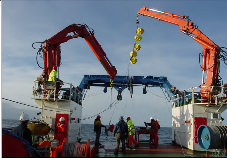
The two cranes working in tandem provide an excellent capability for mooring deployment and recovery.
