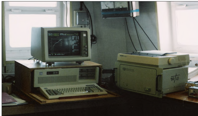
An RD Instruments acoustic Doppler current profiler had been installed on Discovery earlier in the year, here the display shows the acoustic backscatter profile in white with the E/W, N/S current profiles in green and yellow.
