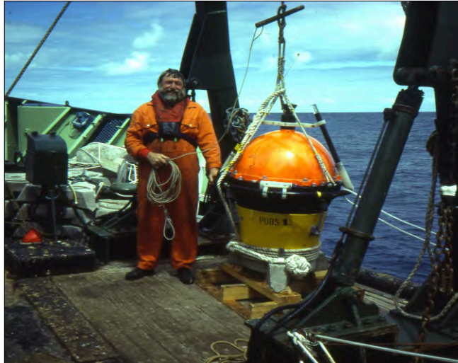
Bosun Frank Smith ready to deploy the OBS from the foredeck 'A' frame. He holds the line to the 'no-load' release pin between the ship's lowering cable and the OBS rope bridle.
