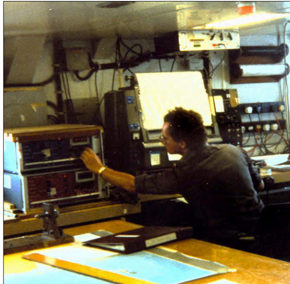
David Billett at the Mufax echo sounder console setting the Deck Unit for the acoustic Net Monitor.
