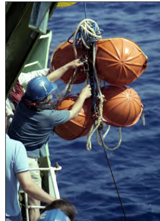
John Swallow and Bob Wallace look on as John Cherriman (in blue) and Ian Waddington (in white) handle the glass buoyancy spheres of a deep-sea mooring.
