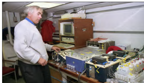
Phil Nightingale (top) with his apparatus for measuring the biogenic gas dimethyl sulphide and Bob Head with the nutrient autoanalyzer.
