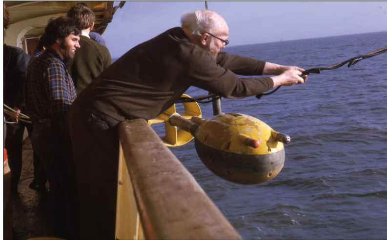
John Swallow with the towed echo sounder fish with John Moorey's temperature and salinity sensors. To the left is Malcolm "Mac" Harris.
