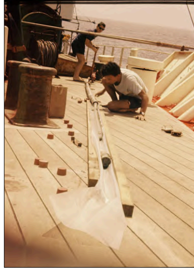
Bob Whitmarsh and Bob Belderson extruding sediment from a gravity corer
