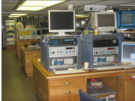
Left: the salinometer in use in the Constant Temperature Laboratory. Above: the CTD control station in the Main Laboratory.
