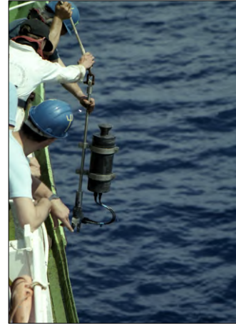
Ian Waddington, John Cherriman and (probably Len the Carpenter) bring an Aanderaa current meter onboard, followed by an IOS acoustic release (right).
