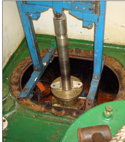
The phased array transducer for the acoustic Doppler current profiler in its transit case, and then in place on the inside of the ship's hull. After the transducer has been put in place, the blue frame is removed, and the green top hat, bottom right, is bolted over the top.
