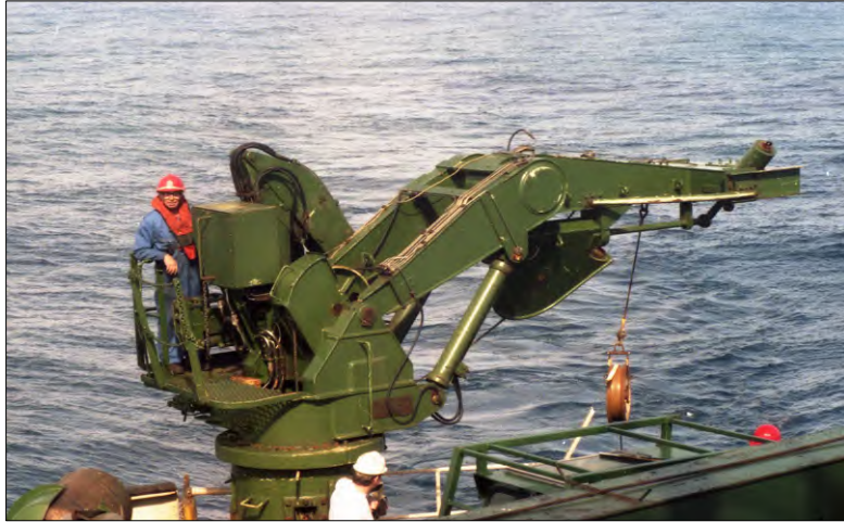
Roy Wild atop the Schat Davit from which the towing block for the SeaSoar was hung.
