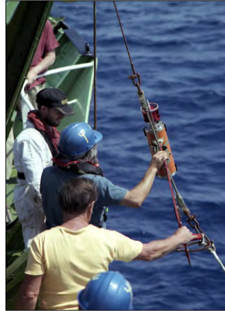
Ian Waddington, John Cherriman and (probably Len the Carpenter) bring an Aanderaa current meter onboard, followed by an IOS acoustic release (right).
