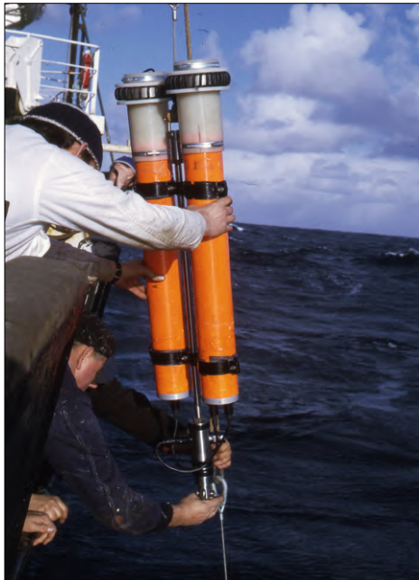
Nickel scroll acoustic transducers atop a pair of acoustic releases.
