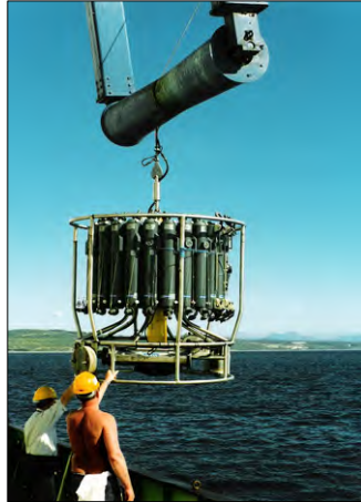
The lowered Doppler profiler surrounded by a rosette of 24 ten litre bottles; the CTD lies horizontal. The tow-fish at right carried transducers at 38, 120 and 200 kHz for the EK500 echo-sounder.
