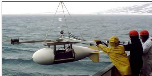
Doug Bone (in white) and colleagues deploy the towfish carrying 38kHz and 120kHz transducers for the EK400 krill echosounder.
