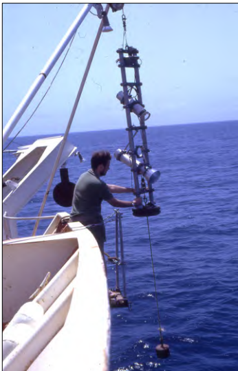
Launching the underwater camera developed by Tony Laughton and colleagues (left) with an image of volcanic boulders about 1ft diameter on a slope at about 2000 m depth near the centre of the Carlsberg Ridge.
