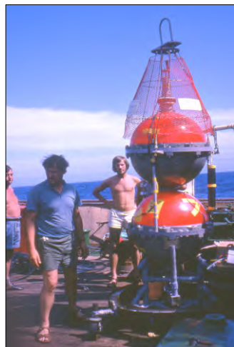
Left: Len Cromwell (Carpenter), Tim Francis and Peter McKeith with an IOS Blacknest Ocean Bottom Seismograph; instrument-ation in the bottom sphere, the top sphere providing buoyancy
