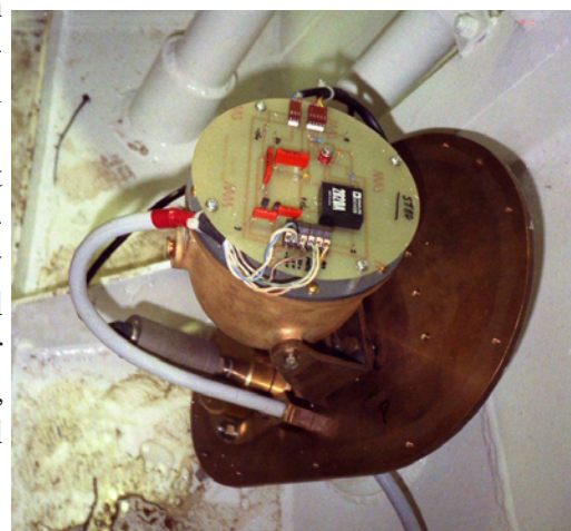
One of the SBWR transducer assemblies bolted to the hull of the Norwegian weather ship Polar Front . The electronics interface card sits atop the brass bowl housing the gimballed accelerometers. The shut-off valve is seen within the bight of the grey cable.
